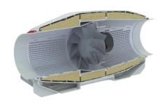
The diffuser, the specially profiled impeller and the directing vanes at the outlet of the fan casing distribute air flow in such a way as to attain the best combination of high performance and high pressure at low noise level.
