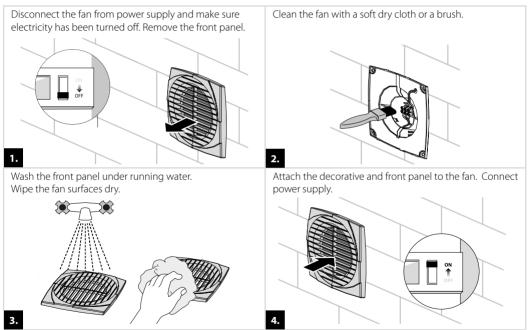
CAUTION! Do not allow water or liquid come into contact with electric components!
