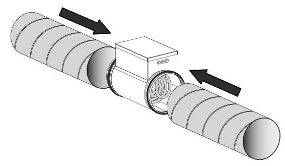
The heater is designed for internal installation into air ducts in the horizontal or vertical position. In a horizontal position the connection box must face upwards. Permitted deviation up to 90 °C. The heater must not be mounted with the connection box suspended downwards (risk of condensate leaking and short circuit of power grid).
