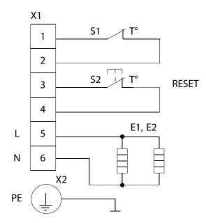
WIRING DIAGRAM OF THE HEATER WITH THREE ELECTRICAL HEATING ELEMENTS AND SINGLE-PHASE POWER SUPPLY
