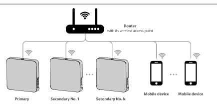
If the Wi-Fi router capacity is not enough to connect a required number of the units, you may use an extra wireless access point to connect the other the unit. Several Master units can optionally be connected to the network for arranging a zone control.
