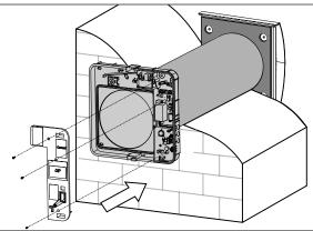
10. Install the cartridge or the regenerator unit and the fan unit into the air duct as figured below and connect the connector to the board as shown by the arrow.
