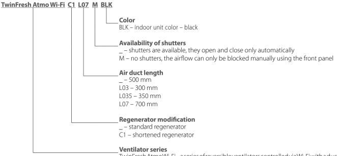
$Twin Fresh Atmo Wi-Fi-a series of reversible ventilators controlled via Wi-Fi with a duct diameter of 160~mm and a nominal capacity of 50~m^3/h$
