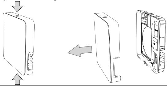
6. Remove the three retaining screws from the controller cover to enable access to the terminals. Route the power wires through the appropriate cable glands.
