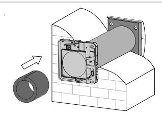
11. Install the front panel of the indoor unit.
