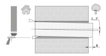
Install the duct into the wall with a slope.
