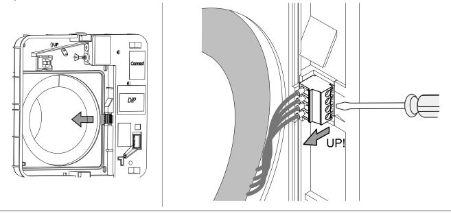
3. Remove the sound-insulation material from the duct, then remove the cartridge or the fan unit and the regenerator unit.
