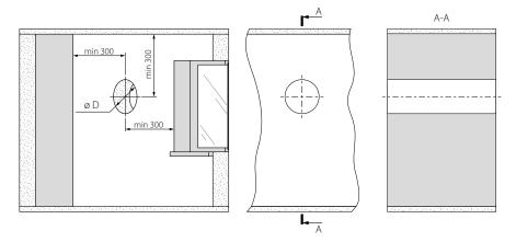
2. Insert the air duct in the wall. For ease of installation use the mounting wedges included in the delivery set. The air duct end must protrude for the distance A that enables installation of the outer ventilation hood. The overall dimensions of the outer ventilation hood, the outside protrusion length of the air duct A and the mounting sequence of the hood are stated in its installation instruction.
