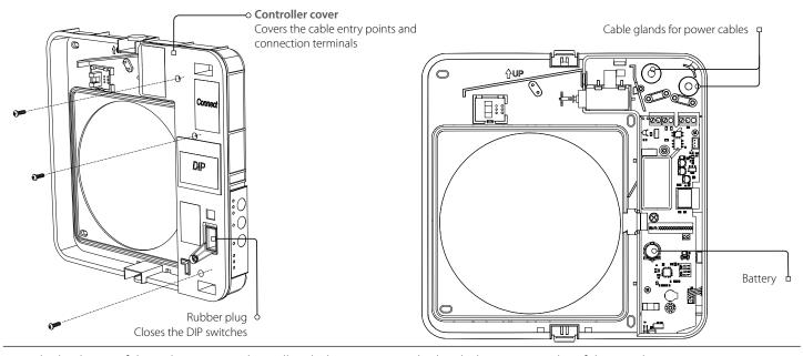
7. Fix the back part of the indoor unit on the wall with the screws supplied with the mounting kit of the ventilator.
