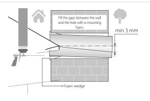
Install the air duct with the minimum slope of 3 mm downwards to the outer wall side using the polystyrene wedges. Fill the gap between the air duct and the opening with mounting foam.
