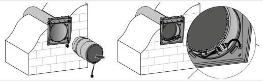
6. Mount the front panel of the indoor unit and fix the outer ventilation hood.
