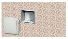
The fan casing is mounted during construction works. Electric wiring for connection of the VNV-1A(E) 80 ventilation unit is led out through a special hole in the casing. The front panel is covered with the protective cardboard plate supplied with the unit to avoid damages or contamination during finishing works in the room. After finishing the works the protective cardboard plate is removed and the VNV-1A(E) 80 ventilation unit is installed into the casing that is connected to the wiring.
